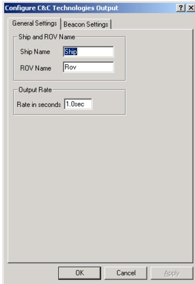
The first tab of the dialog allows you to enter the ship name and ROV name. These must be entered so WinFrog can place their coordinates in the correct location in the telegram. Also enter the output rate. The data will be output at this rate regardless of whether new beacon data has become available. However, data will only be output if there are valid positions for both the vessels – i.e. neither vessel has a position alarm.
